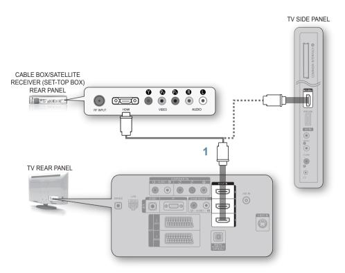
1. Connect an HDMI Cable (Not supplied) between the HDMI IN (1, 2, 3 or 4) jack on the TV and the HDMI jack on the Cable Box/Satellite receiver (Set-Top Box).
